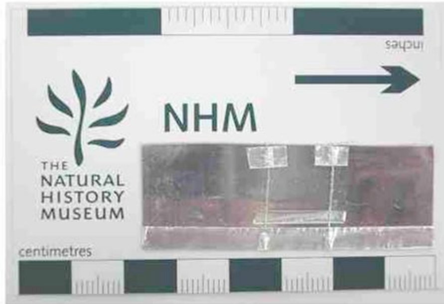
Test sample with two Sn wires.
