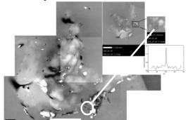
Figure 1 Montage of both TEM and STXM images of Stardust particle FC12,0,16,1,3 Black circled area is where carbon XANES spectra were obtained and white circled area is where EDS and electron diffraction identified a possible carbonate.
