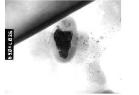
Figure 3 TEM image of a carbonate (dark area) surrounded by a SiO2 layer. The field of view is 1.5 microns.
