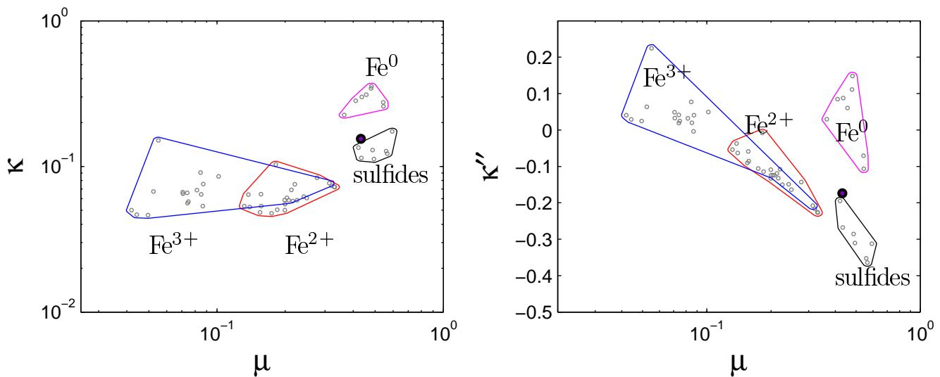
Because of strong degeneracies between Fe-XANES absorption spectra of minerals within a given oxidation state (metal, sulfide,  $\text{Fe}^{2+}$ ,  $\text{Fe}^{3+}$ ) specific mineral identifications are not reliable. Treat these analyses as indicative but not definitive.
