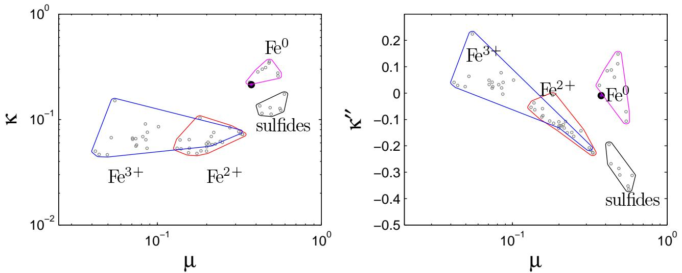
Because of strong degeneracies between Fe-XANES absorption spectra of minerals within a given oxidation state (metal, sulfide,  $Fe^{2+}$ ,  $Fe^{3+}$ ) specific mineral identifications are not reliable. Treat these analyses as indicative but not definitive.
