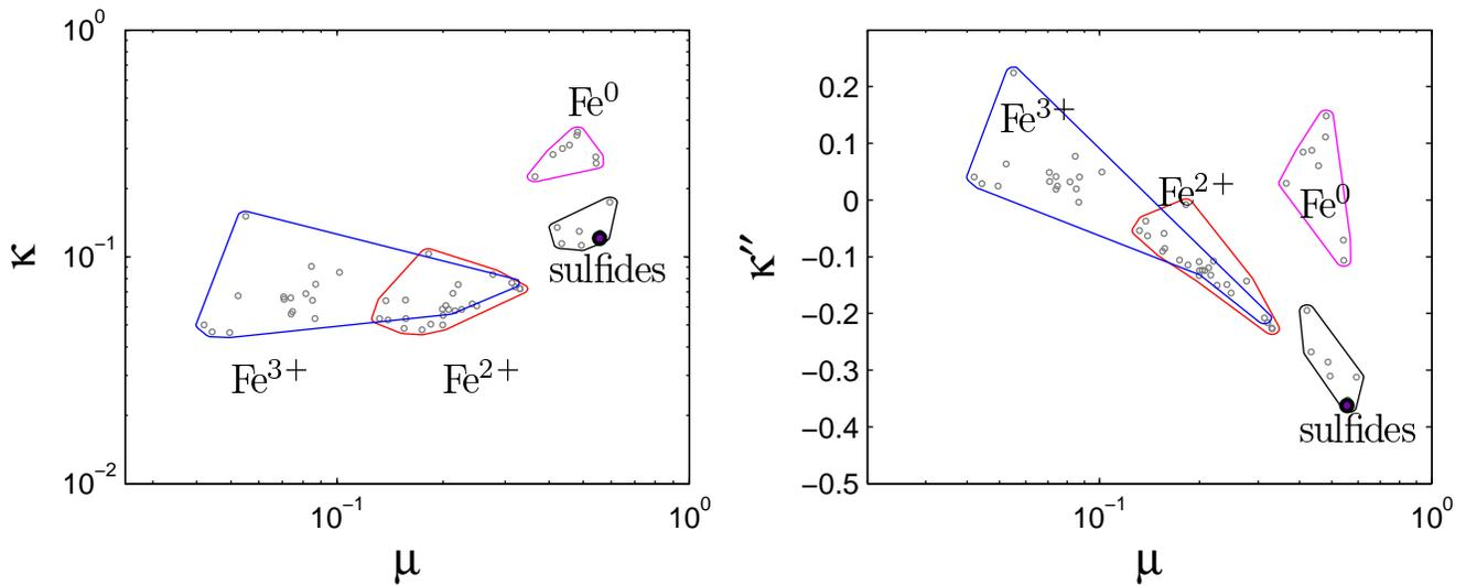
Because of strong degeneracies between Fe-XANES absorption spectra of minerals within a given oxidation state (metal, sulfide, Fe<sup>2+</sup>, Fe<sup>3+</sup>) specific mineral identifications are not reliable. Treat these analyses as indicative but not definitive.
